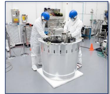
*The fully integrated cryostat will keep LSST's camera chilled to a cool -150°F*
